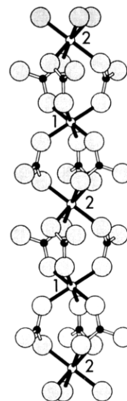
Figure 2. Drawing of an individual chain containing Sc1- and Sc2-centered distorted octahedra bridged by \text{BO}_3 groups.
